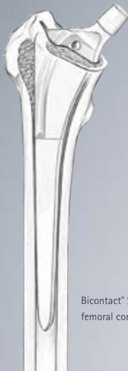
Bicontact® S for normal femoral conditions
