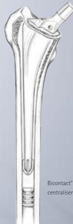
Bicontact® stem position with centraliser and intermedullary plug
